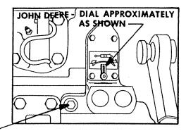
Typical plug for surplus relief flow line. Check carefully that it enters the reservoir before using. Note that the location varies with different tractor makes and models. A John Deere Tractor is shown.
